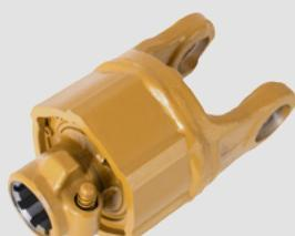
OVERRUNNING CLUTCH is designed to protect against over-torque moment caused by inertia of agricultural machine, arising during braking or complete stop of tractor. One way clutch transmits torque in one direction only due to engagement of ratchets on clutch housing, in the opposite direction, clutch is turned freely. Standard overtaking clutch is a right-hand rotation clutch.
