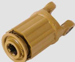
In radial pin couplings, spring-loaded pins fit with the corresponding grooves in housing. Spring compression force coupling determines transmitted torque.
