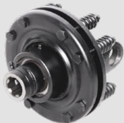
It is used in agricultural machinery operating with a constant excess of torque that must be overcome without interrupting the transmission of torque and the movement of the machine. The friction backstop transmits torque by means of friction plates located between the flange yoke and the clutch hub.
