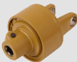
In case of overload, clutch switches off without causing any damages (as e.g. in ratchet, friction or shear bolt limiters). When resistance is overcome, clutch is automatically switched on and torque is transmitted.
