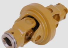
Wide-angle joint is mounted on PTO shaft. It ensures its steady operation and enables PTO shaft to work at an angle up to 80 degrees.
